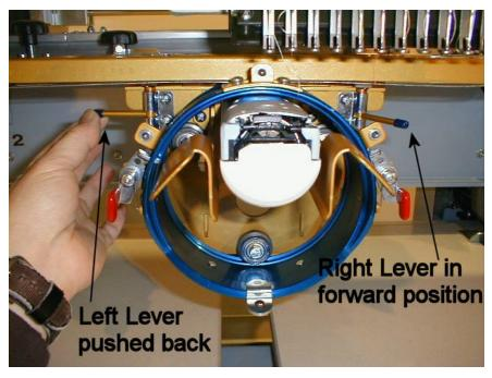
7. Push the two (left and right) cam lock levers all the way back, towards the back of the machine, as shown in the photo above.
