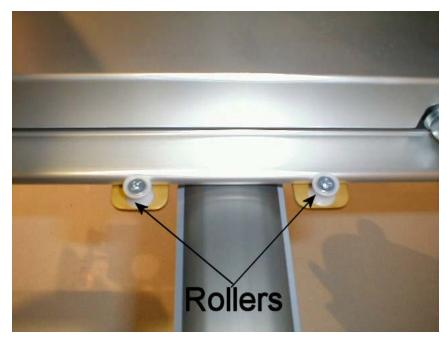
Note: The white rollers should snap over the back of the pantograph
