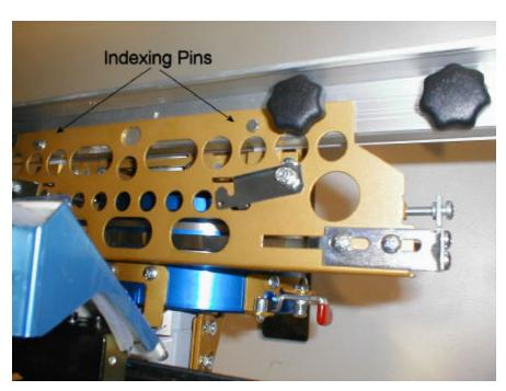
5. Lift the bracket over the pantograph and place it under the indexing pins. Tighten the knobs.
