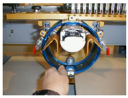
6. Pushing the cap frame drive unit from the bottom, push it all the way back until the cap frame snaps into place on the back of the pantograph.
