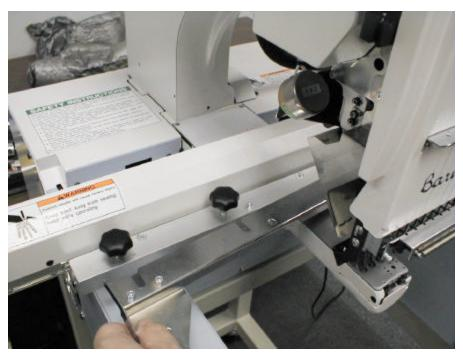
1. Remove the Panto Hoop Arm Stay from the top of the pantograph.
