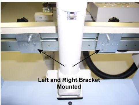
3. Attach the Left and Right Mounting Brackets using the (4) M5 x 10mm Flat head screws, as pictured.
