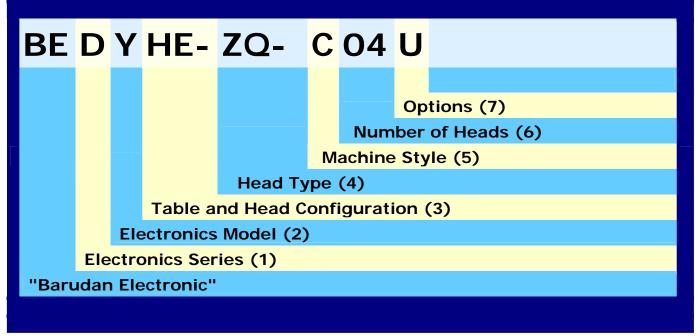
ELECTRONICS (SERIES AND MODEL) (1) & (2) Barudan machines typically have an "AUTOMAT" (control box above the table top) with displays and switches, and a "Driver Box" located underneath the machine that powers the motors and solenoids.
