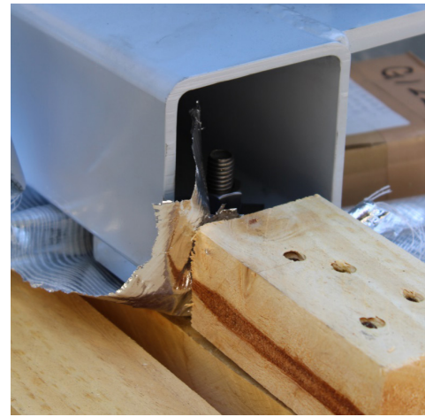
10. The machine is bolted to the bottom of the crate. Remove the nuts from the top, and push the bolts through the bottom of the crate. Note the machine wheel is bolted upside down to the machine chassis. Remove the wheels and nuts. Set aside for now.
