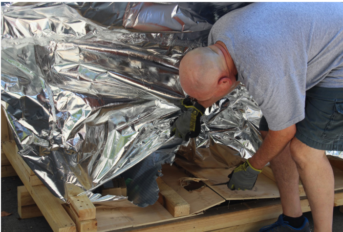
8. Carefully cut the moisture barrier as close to the bottom of the machine as possible. Remove the moisture barrier and discard.
