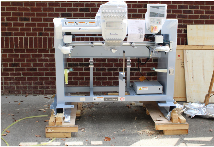
13. With the center portion of the pallet removed, the machine will be sitting on the remaining ends of the pallet.
