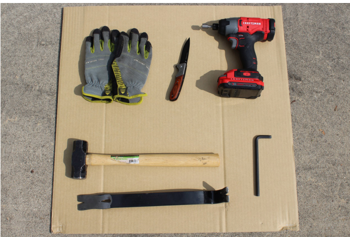
3. The tools needed to uncrate the machine: drill with 10 mm socket, hammer, pry bar, knife and gloves. If no forklift is available to lift the machine off the pallet, a chainsaw or reciprocating saw will be needed. A ladder is also recommended to remove the top bolts from the crate.
