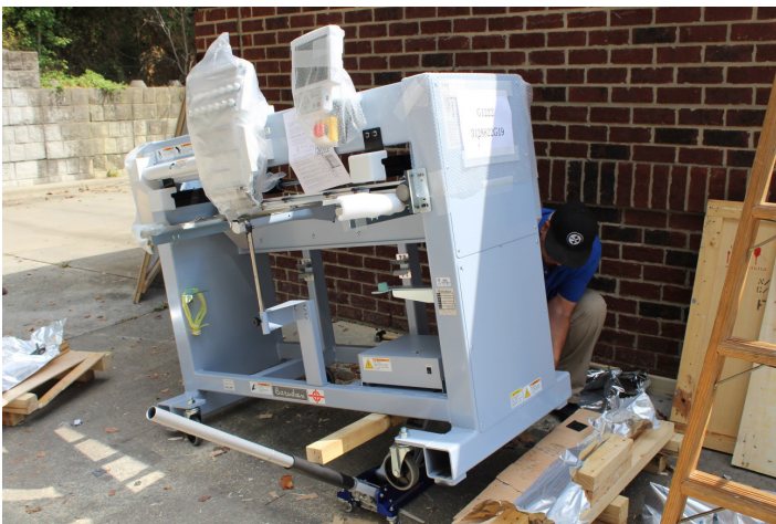
15. Do the same on the opposite side of the machine. The machine is on the wheels and ready to be moved into position.
