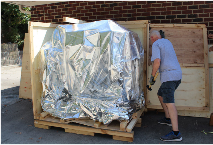
7. The machine is bolted to the pallet and packed in a sealed moisture barrier.
