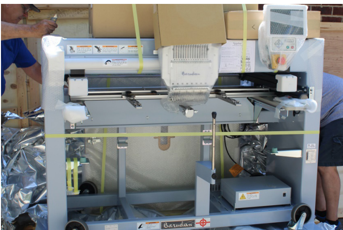
9. With the moisture barrier removed, cut the yellow banding and set aside the accessory boxes.
