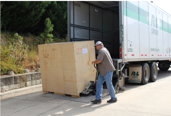
2. The machine is lowered to the ground by a liftgate and moved with a pallet jack, which is provided by the trucking company.
