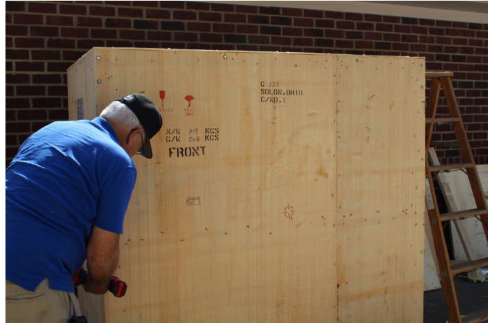
4. First, remove all of the lag bolts from the front of the machine crate with the battery drill and 10 mm socket.
